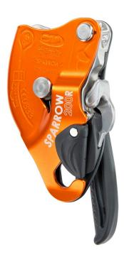
Self-braking descender for rope work has been developed for high workloads. It allows the operator to lower themselves on the working line, to position themselves on the working line and to ascend the same rope. It is ideal in the event of assisted lowering of two people with the device installed at the anchor (the operator lowers the rescuer and the person being rescued) or for simultaneous lowering of two people (rescuer lowers themselves with the injured person).
